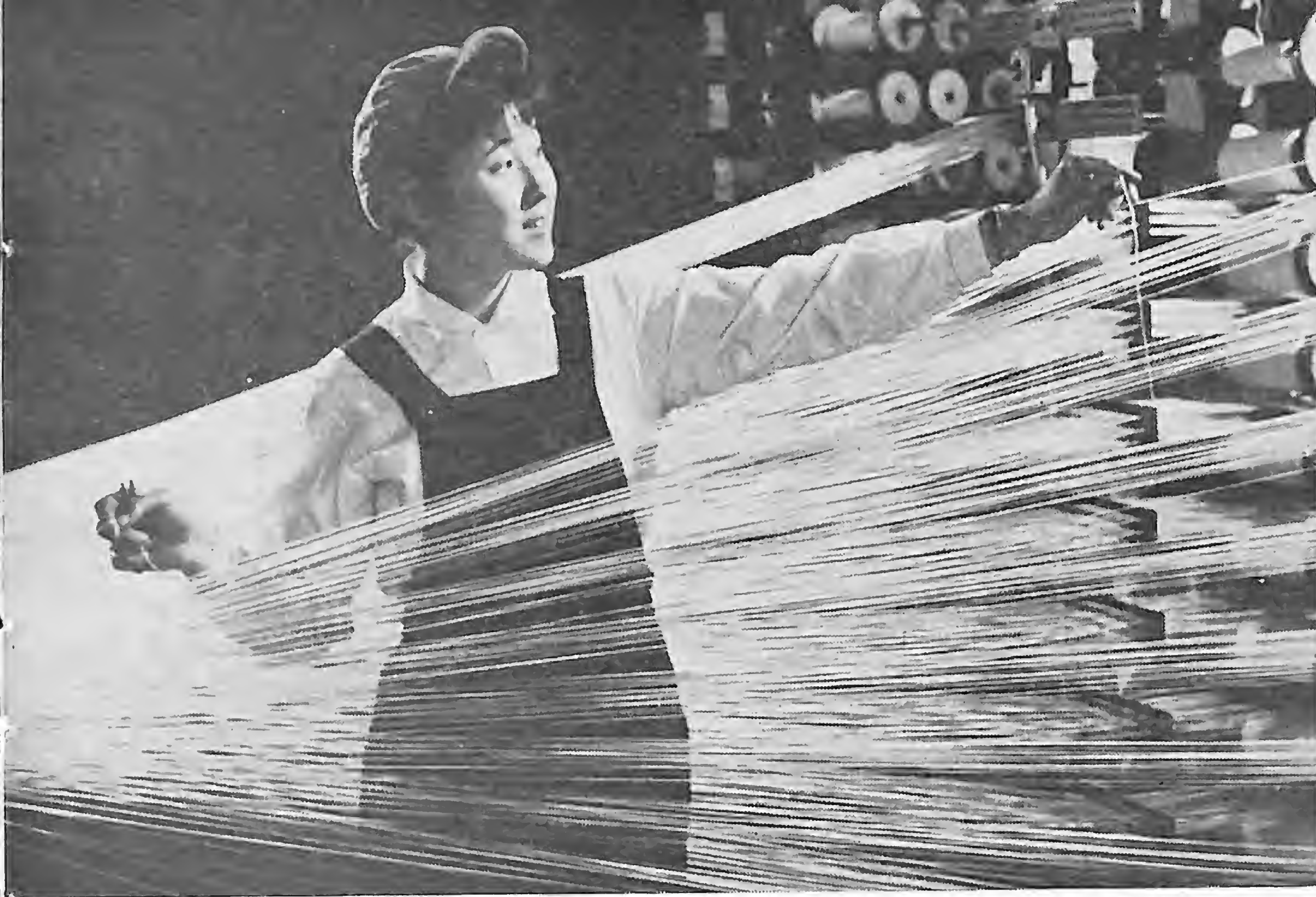
A worker of Hui nationality operating a warping machine at the Yinchuan Cotton Mill, Ningsia Hui Autonomous Region, one of many modern cotton mills set up in national minority regions.
